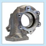
Cutting data:  $v_c = 140 \text{m/min}$  $a_p = 2.5 \text{ mm}$
